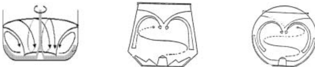
FIGURE 5 High-shear Mixer-granulators with Different Mixing Chamber Design (Gaillard, 1990, Ramaker, 2001).
